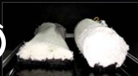
Cross sections placed in spilled oil. SpillBoa® Boom (left), competitor boom (right).
